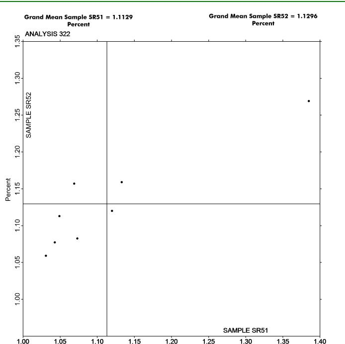
**Percent** If fewer than 20 laboratories are included in an analysis, a control ellipse will not be drawn on the two-sample plot.
