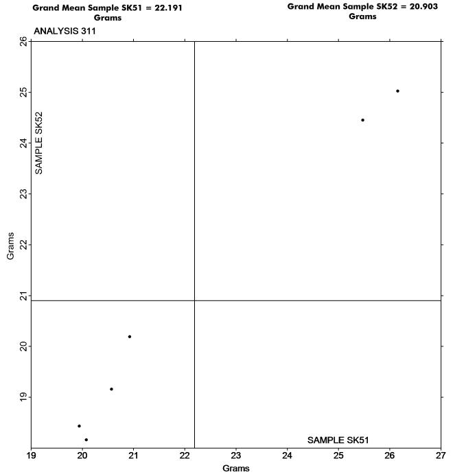
If fewer than 20 laboratories are included in an analysis, a control ellipse will not be drawn on the two-sample plot.
